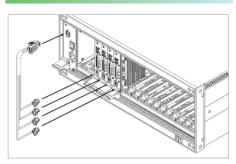
One A330101 power supply supports up to 200W (4 pcs of 33010 digital IO cards)
