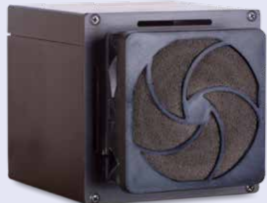
The GigE Cubes automatically include a cooling fan as shown above. The fan is available as an option on the standard Cubes and is only recommended when total Cube power dissipation will exceed 15 Watts for the smaller Cube or 24 Watts on Cubes with six I/O slots. The fans are thermostatically controlled and only turn on when the internal temperature of the Cube reaches roughly 35 °C.
