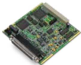
DNA-series boards such as this DNA-AI-207 are used with Cube, DNA-series and UEINet chassis.
