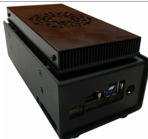
Illustration 4: Rear view of SBC-Nano aluminum chassis, shown with optional fansink installed. Substitute cold-plate for fan-sink in conduction-cooled applications.
