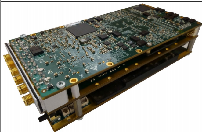
Illustration 3: Bottom view of XMC module, SBC-Nano and mSATA expansion boards.
