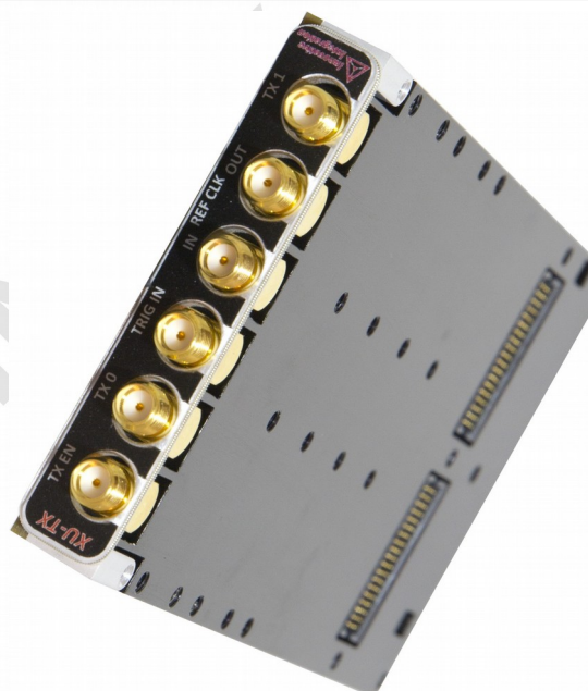
Illustration 2: XU-TX top, with heat spreader installed
